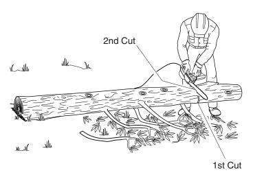
Figure 16 - Bucking Log When Log Is Supported
